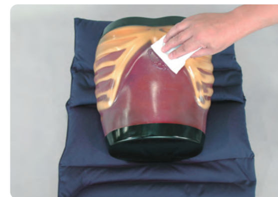
Wipe the remaining gel completely by wet cloth. If remaining gel gets dried up on the body, it may cause scratches and tears on the phantom material.
